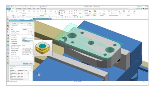
**5-axis milling** – CAM Pro offers highly flexible 5-axis programming functions combining highly automated elements for tedious tasks such as geometry selection and detailed user control for roughing and precise machining. 5-Axis Roughing allows for greater efficiency and longer tool life when machining complex geometry
